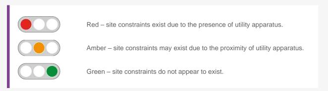
This report confirms to QL-D of PAS 128:2014 - Specification for Underground Utility Detection, Verification and Location. To obtain further detail on utility locations consider site reconnaissance (QL-C), detection (QL-B) and verification (QL-A) as recommended under 'Important Information'.
